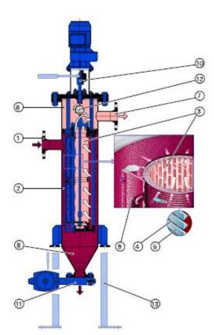
The filtered fluid exits the filter housing at the top opposite the inlet connection. In the AF 95 S version, the integrated preseparator relieves the filter cartridge of coarse and heavy particles by means of a tangential flow around the tube.
