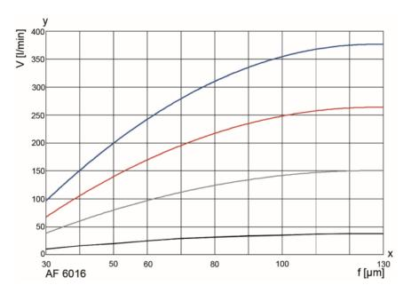
The curves represent the volumetric flow through the entire filter system (filter housing including for example one cartridge) and refer to a differential pressure of 0.3 bar. Specific information about process data is essential for reliable operation of an automatic filter.
